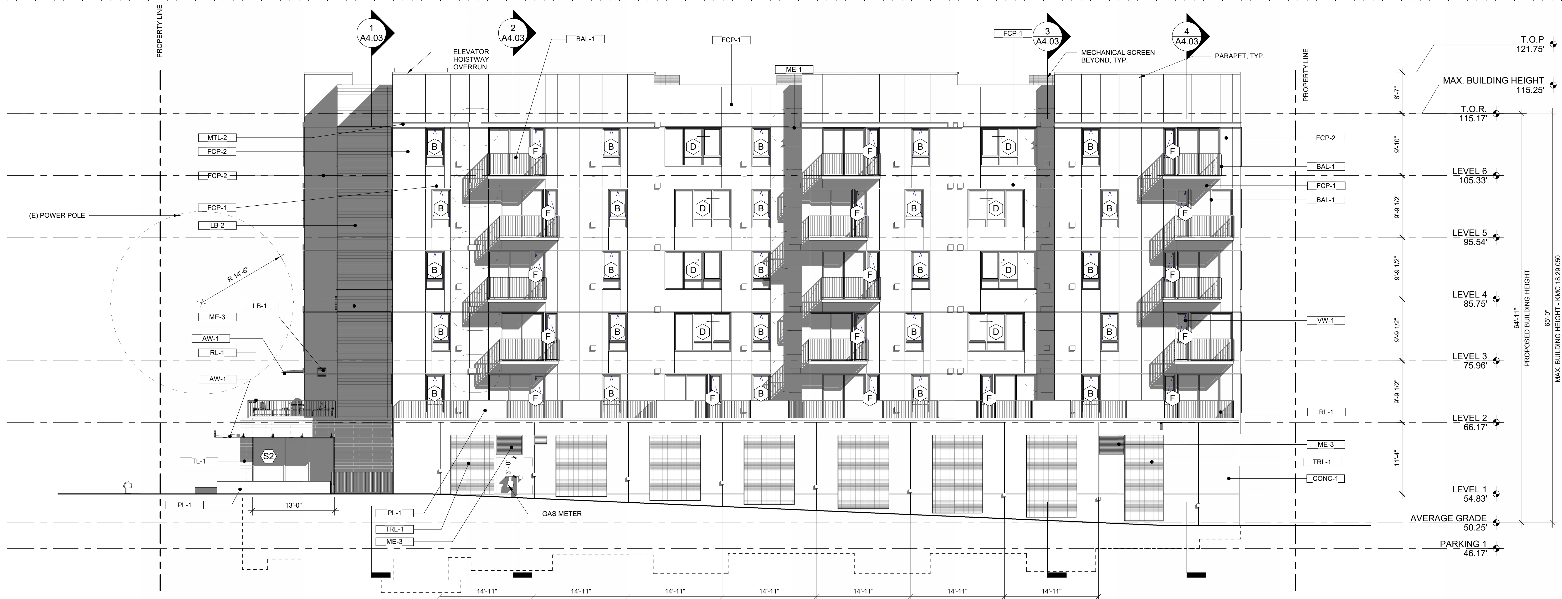
1 BUILDING ELEVATION - NORTH SCALE: 1/8" = 1'-0"
