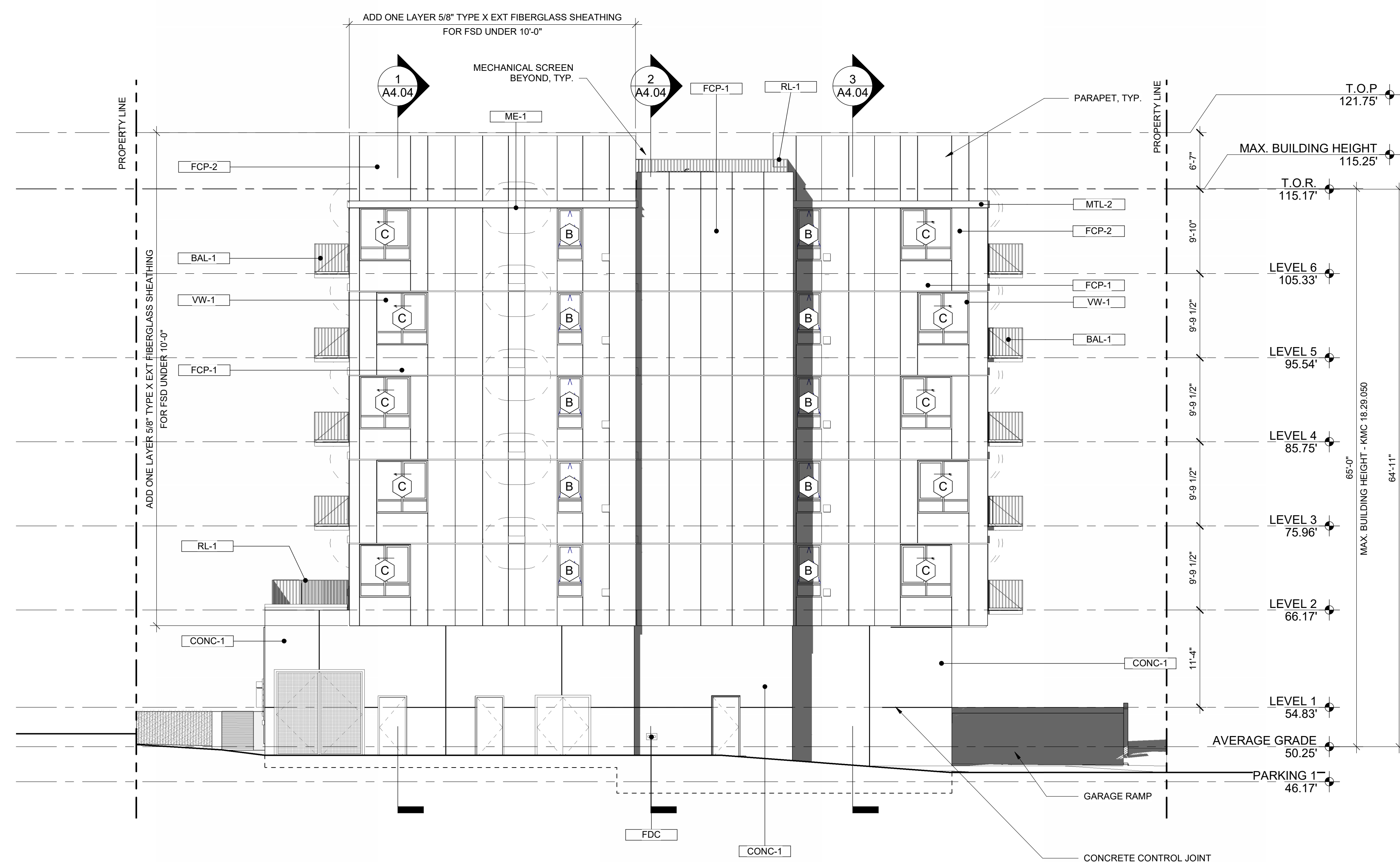
2 BUILDING ELEVATION - WEST SCALE: 1/8" = 1'-0"
